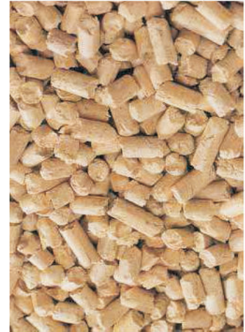
Wood pellets. Made of wood chips after grinding, drying and compression.
