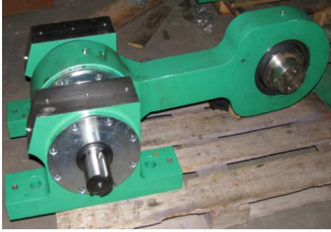
Figure 5 Ready to ship drive rod module – here 1 out of 4 is shown.
