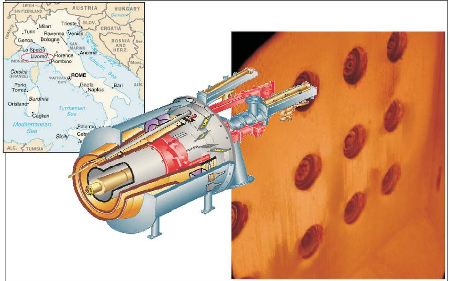
The WR windbox burner units are provided with individual air flow controls and individual flow measurements for airflow balancing. It can be delivered as a coal/oil/orimulsion/gas or biomass burner.
