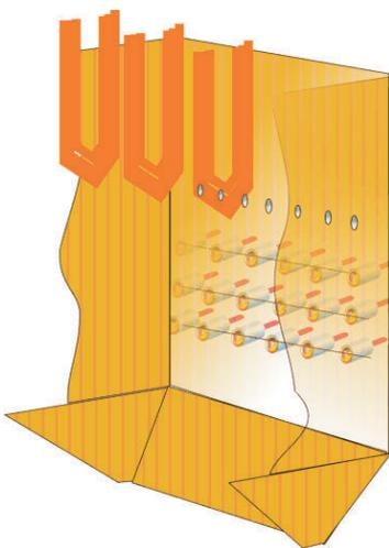
The installation at La Spezia consists of 36 burners arranged in boxer firing, with OFA nozzles above the upper burners on each side of the furnace.
