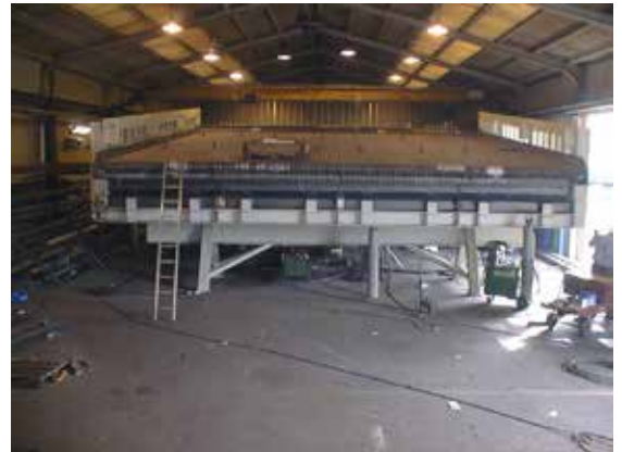
Vibration grate at test assembly in workshop.
