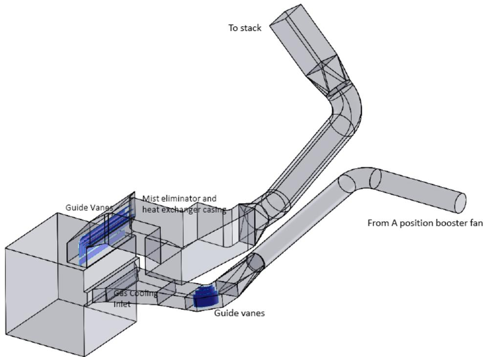
*Figure 4 Sketch of JBR inlet and outlet ducts*
