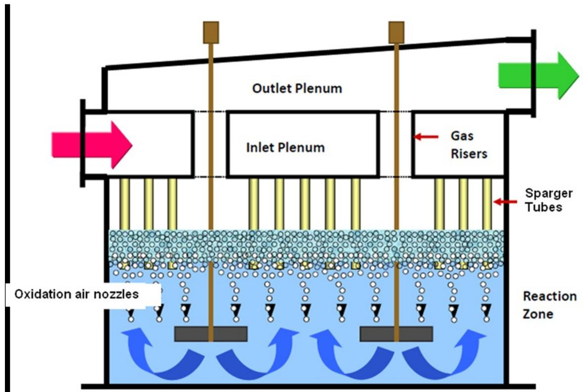
Figure 1 Schematics of the CT-121 Jet Bubbling Reactor
