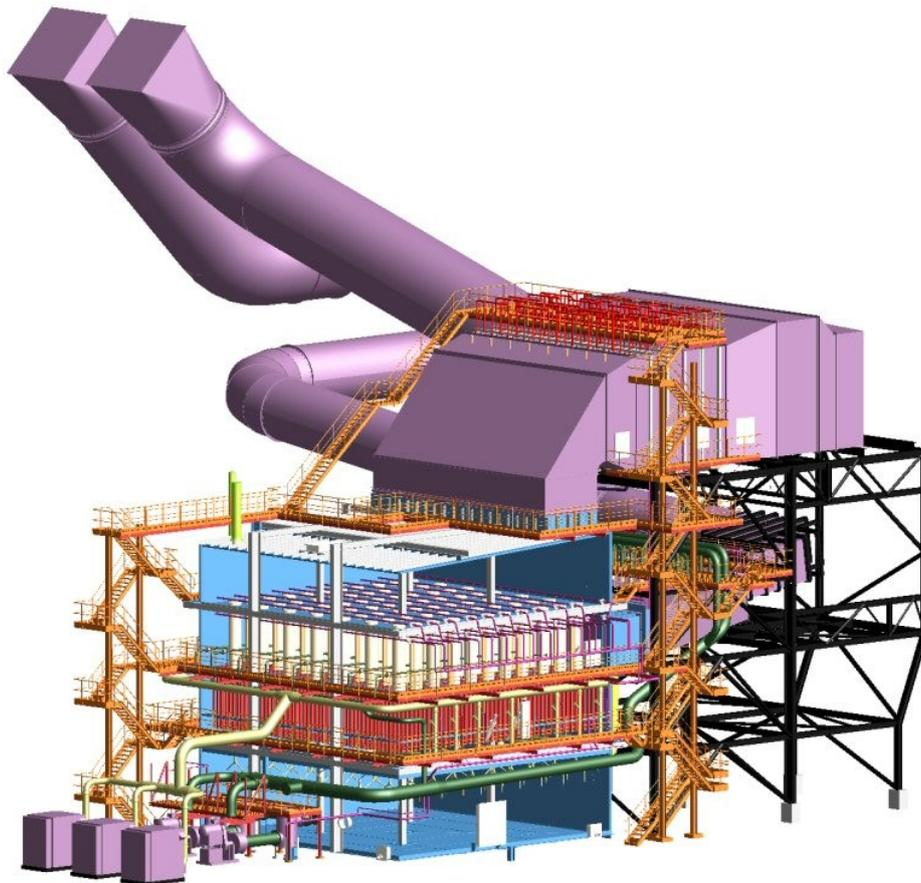
*Figure 3 Cut view of the JBR with auxiliary installations*
