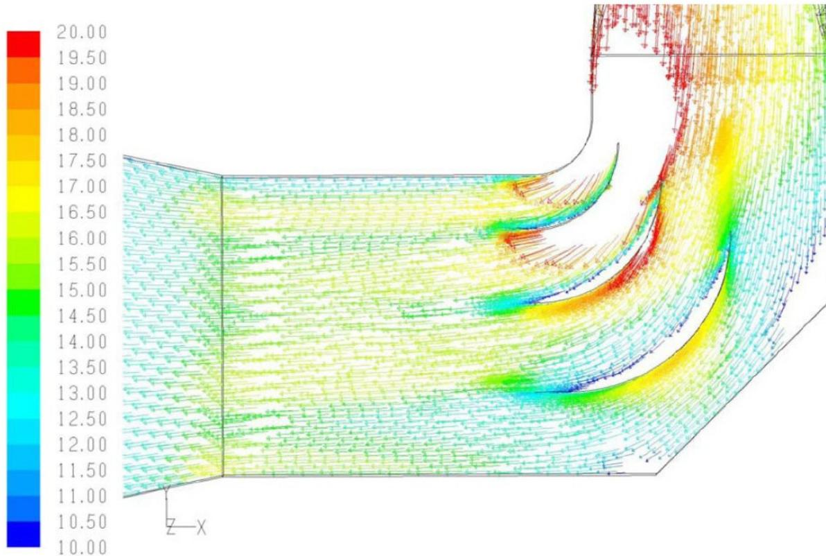
*Figure 5 Velocity plot at the duct centre horizontal plane upstream of the Gas Cooling Section, m/s*
