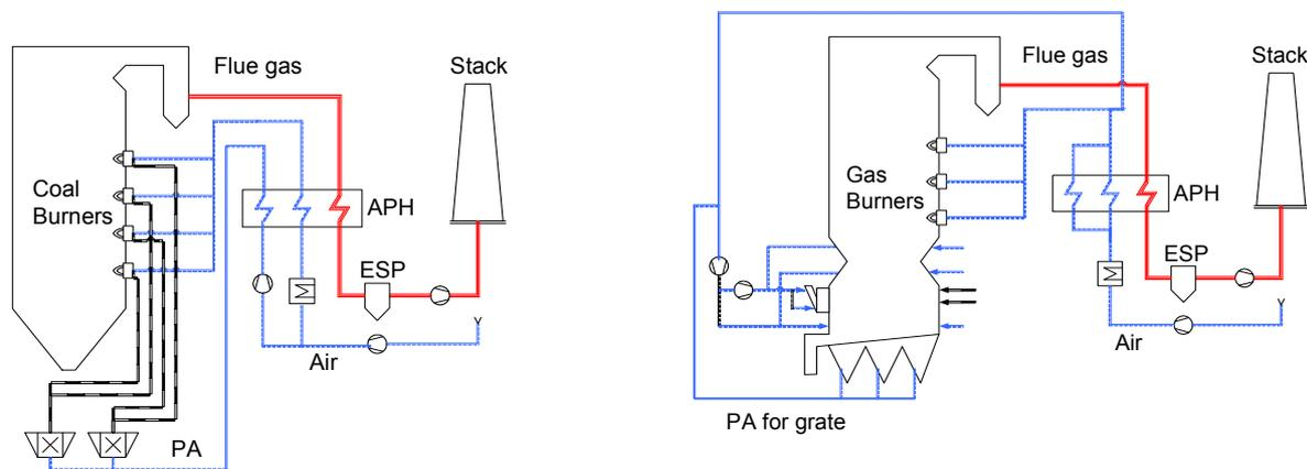
**Figure 2** *Herningværket 1982 with coal/oil (left) and retrofitted for wood chips in 2002 (right).*
