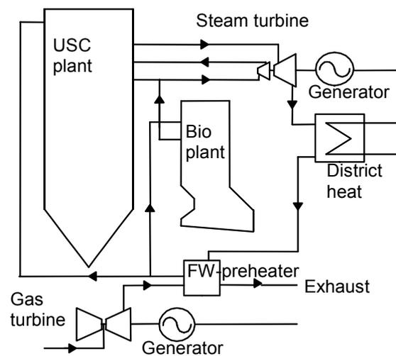
**Figure 3** Schematic view of Avedøre unit 2. The HP-steam from the USC- and biomass-plant are connected and the feed water can be preheated by the gas turbine exhaust gas.
