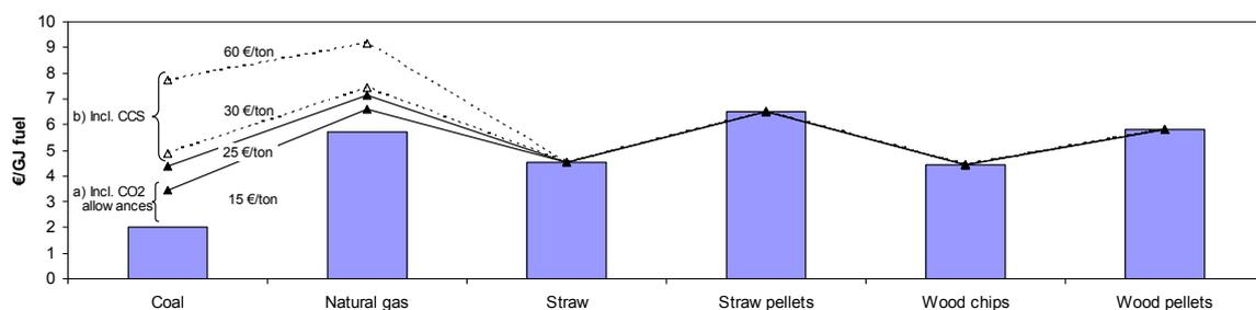
**Figure 1** Fuel price for coal and natural gas are compared with CO<sub>2</sub> neutral biomass fuels. The total price for the fossil fuels are shown in the case of
