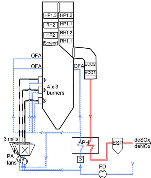
**Figure 2.** Schematic presentation of the steam, fuel, air and flue gas system.
