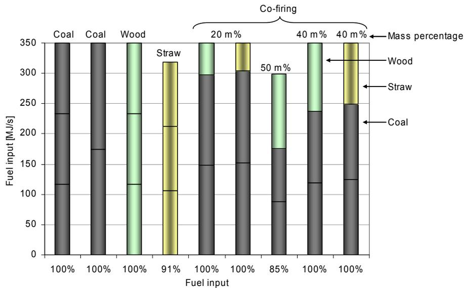
**Figure 4** Mill patterns for various combinations of coal, wood and straw. Typical co-firing will be with one mill on biomass and one or two mills on coal.
