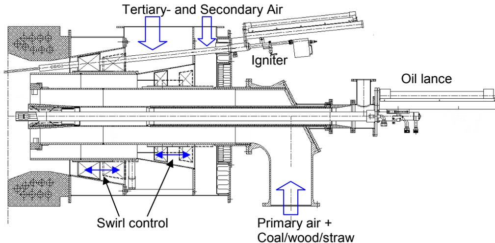
**Figure 3** Coal, oil, wood and straw burner.
