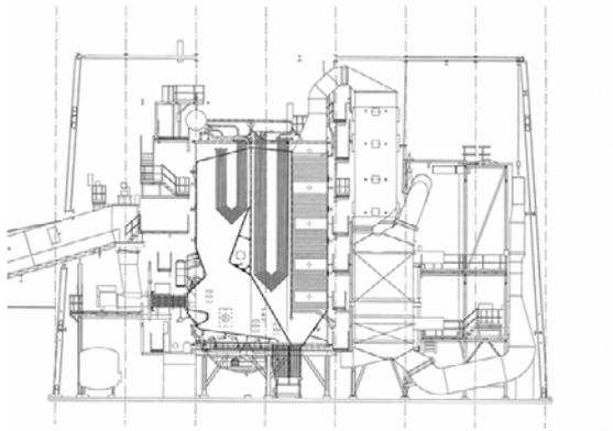
**Figure 5.** Biomass boiler for straw firing.
