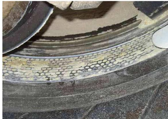
**Figure 13.** Pelletising mill, rotor and matrix.
