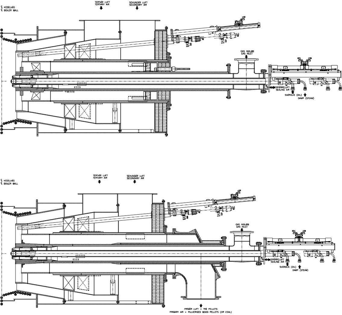
Figure 4. Burner fuel conversion from NG/HFO (top) to NG/HFO/PF (below).
