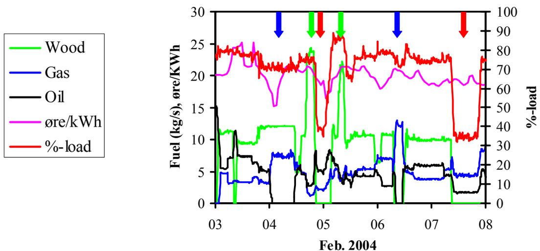
**Figure 16.** Fuel flexibility from the plant record.
