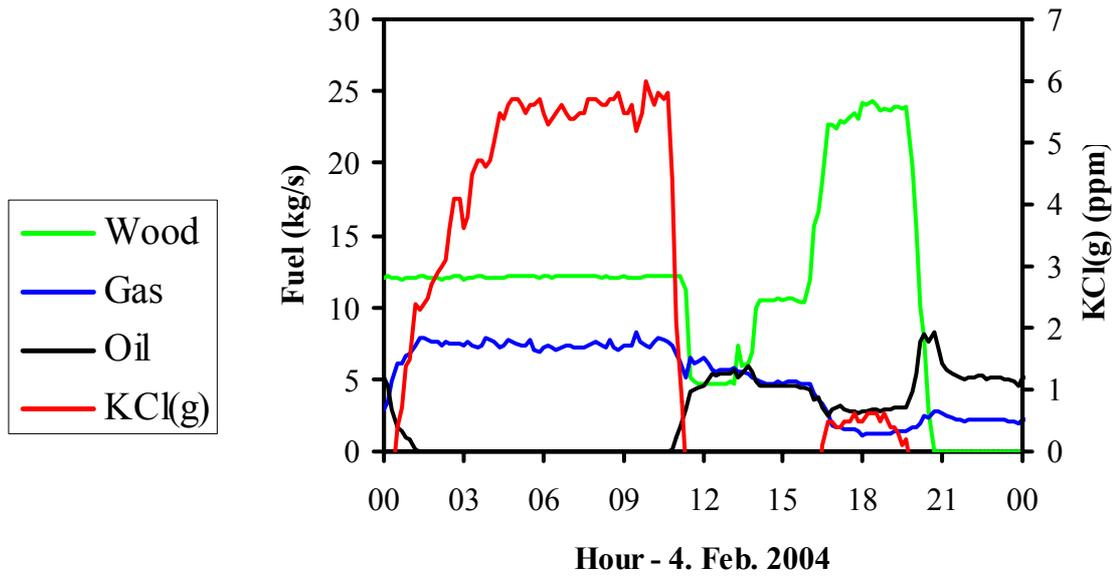
**Figure 18.** Abatement of KCl formation by means of HFO together with the biomass fuel
