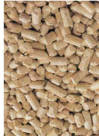
**Figure 11.** Wood pellets. Made of wood chips after grinding, drying and compression.
