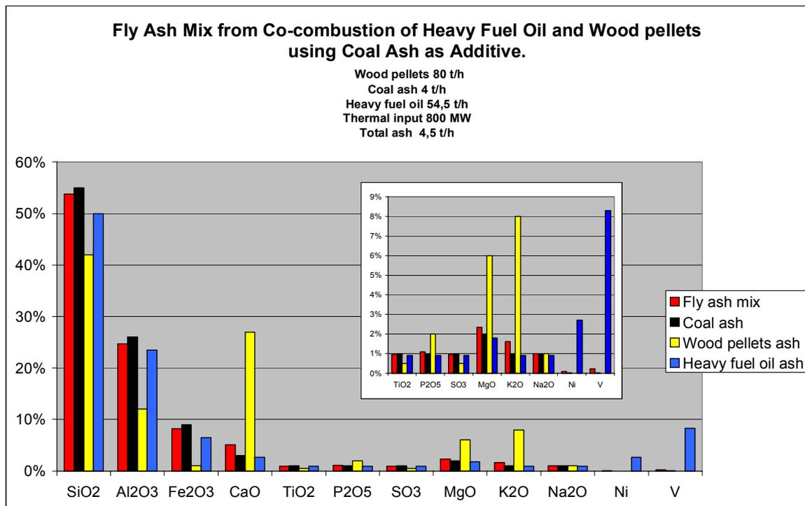
**Figure 17.** Restructuring of the ash from biomass fuel by a cheap additive.
